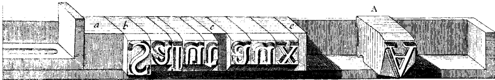
Figure 0-4: A composing stick (from the Encyclopédie of Diderot and d'Alembert).
