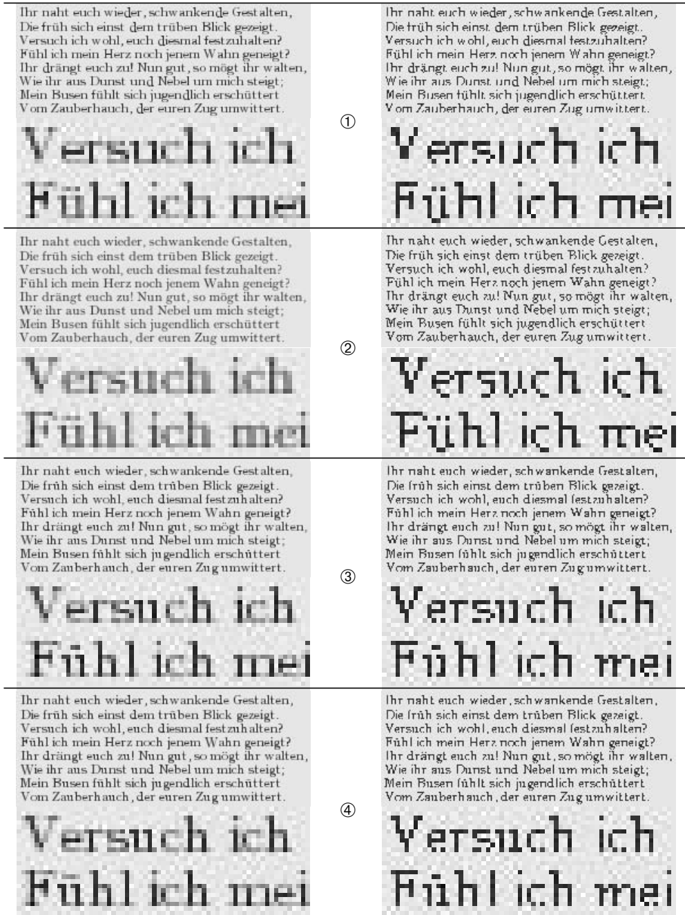
Figure 13-1: A comparison of various optimizations of the rasterization of a PostScript Type 1 font. The font is Monotype Old Style. Left: as rasterized by freetype with gray levels. Right: without gray levels. ① The font's original hints. ② The font without hints. ③ The hints generated by FontForge. ④ The hints generated by FontLab. The text is from Goethe: "Ye wavering shapes, again ye do enfold me / As erst upon my troubled sight ye stole," etc.
